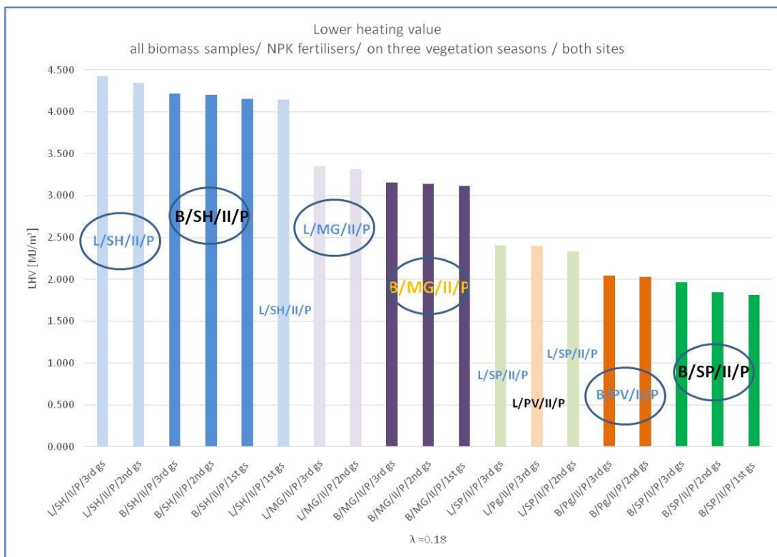
Figure 4 The lower heating value (LHV) all plants treated with NPK fertilizer collected from Bytom and Leipzig new plantations after all three growing seasons
